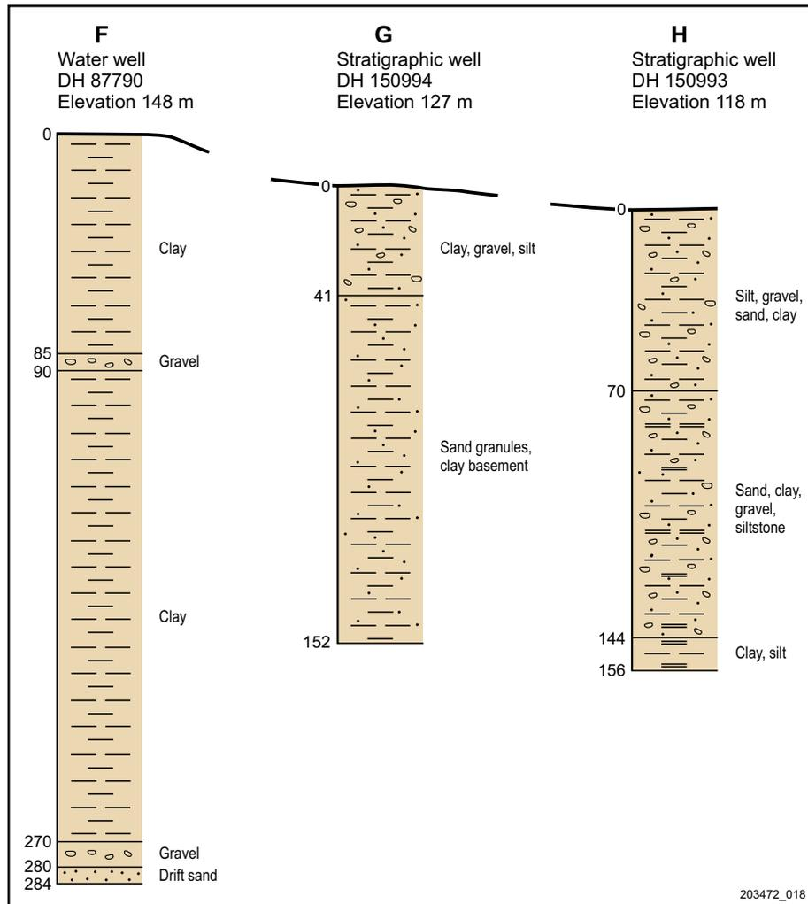
Figure 6 Geological cross-section, drillholes DH 87790, 150994 and 150993 (F, G and H in Fig. 3).
