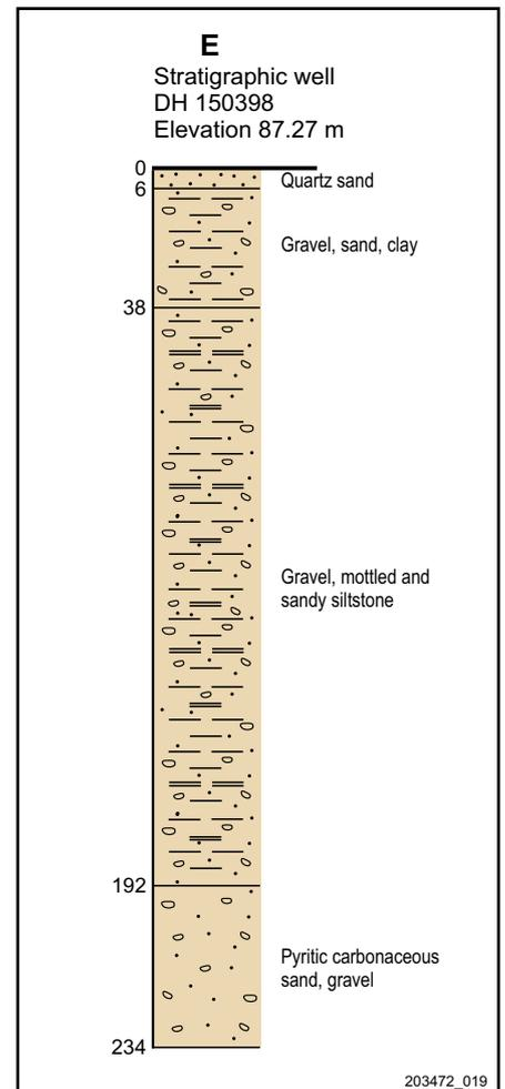
**Figure 5** Geological log, drillhole DH 150398 (E in Fig. 3).
