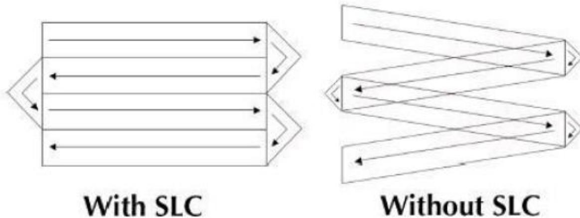
**Figure 3: Diagram explaining the different scan pattern after the SLC failure**
