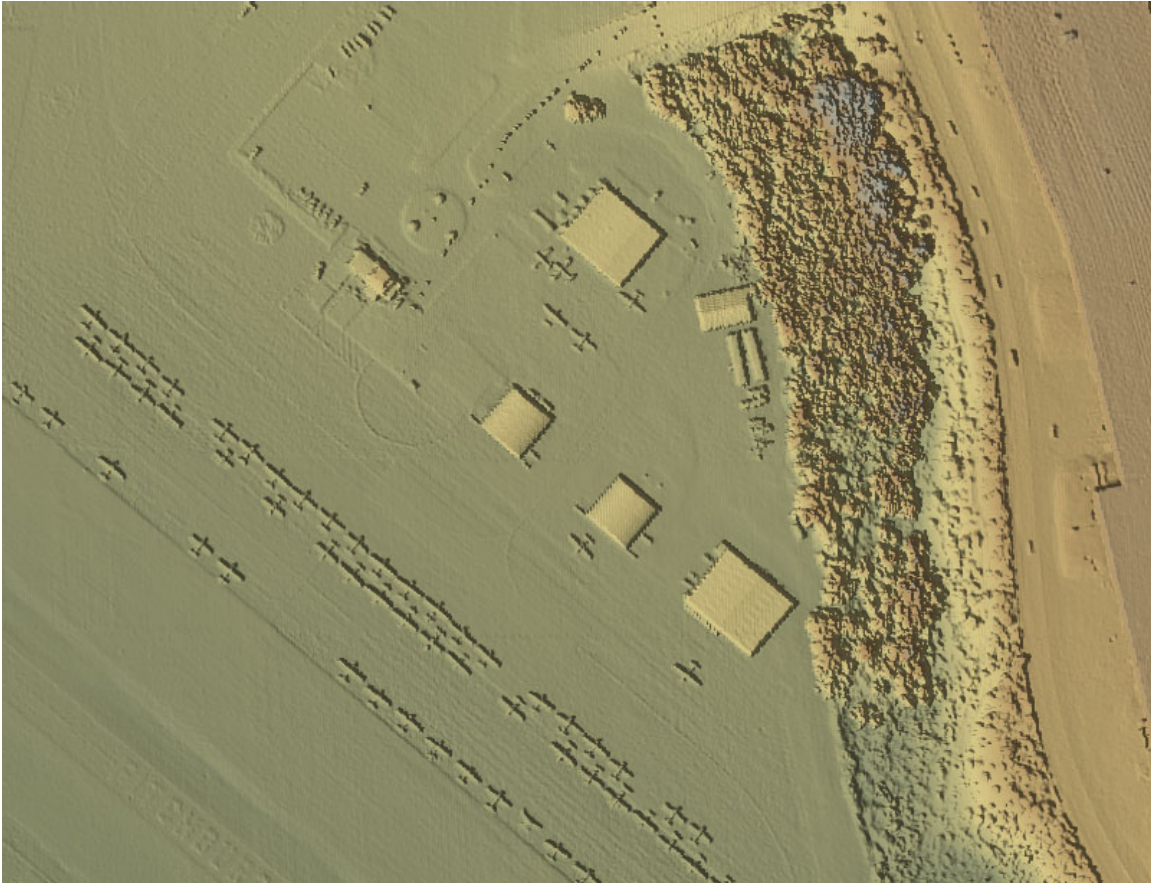
Digital Elevation Model Created from LIDAR Data (one-half meter grid resolution)
